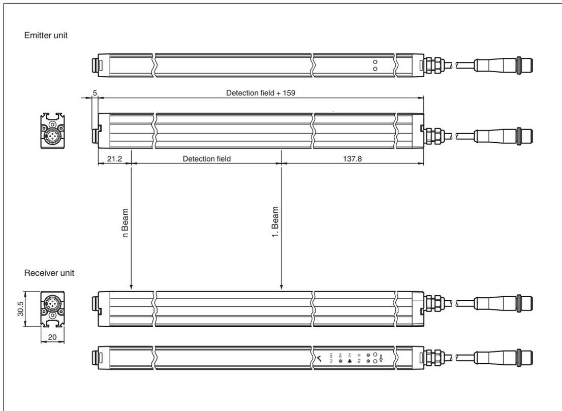
Figure 5.1 Light Grid Dimension Drawing
