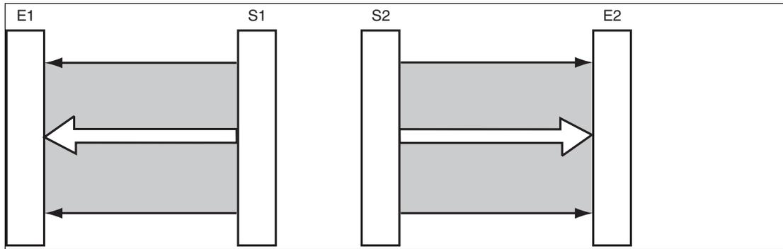
Figure 5.5 Multiple assignment of two pairs of light grids
