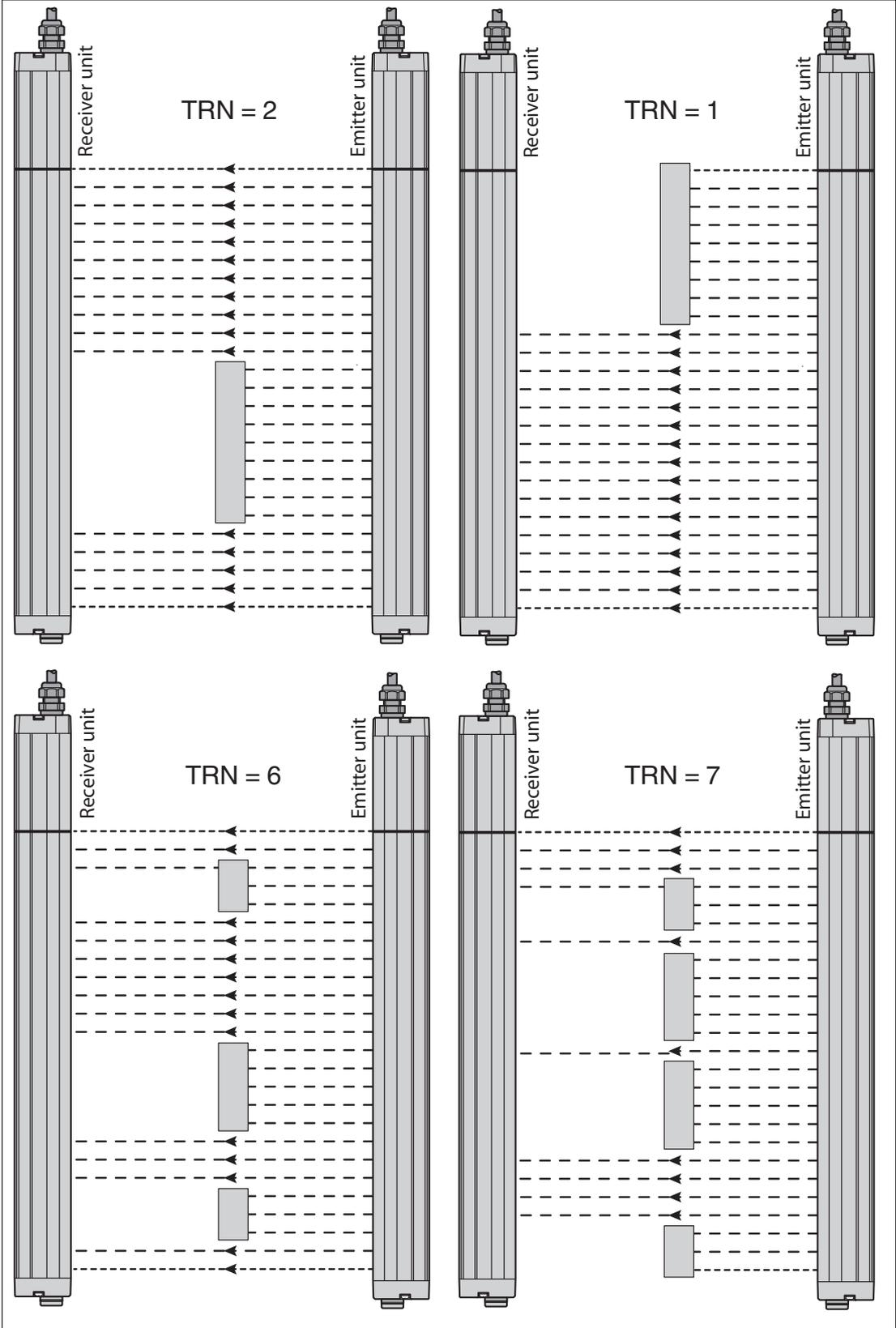
Figure 7.20 Function 30 = Number of transitions from detected to nondetected beams
