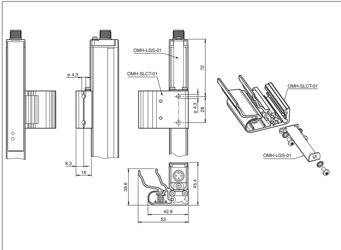
Figure 11.1 Dimensional drawing and fitting mounting accessory OMH-LGS-01
