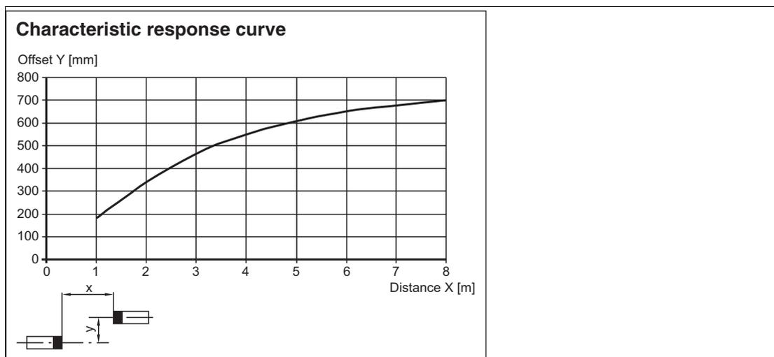
Figure 5.4 Maximum offset between emitter and receiver
