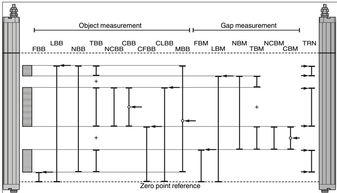
Figure 7.2 Overview of all the Light Grid's Measurement Value Modes
