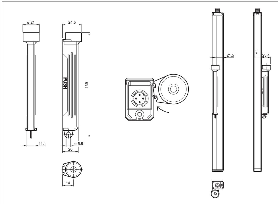
Figure 11.2 Dimensional drawing and assembly of the alignment AA-SLCT-01
