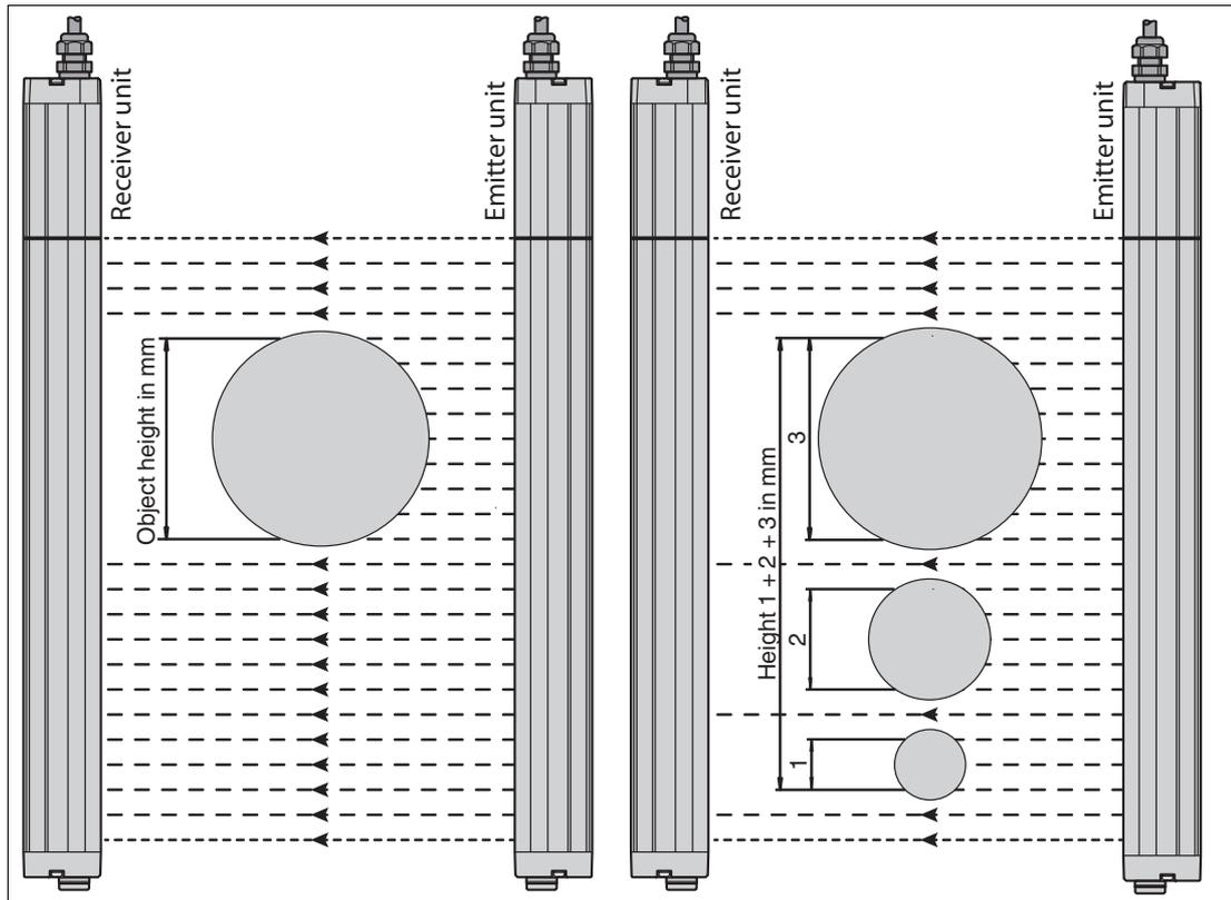
Figure 7.8 Function 3 = Object height as the total height of all partial objects
