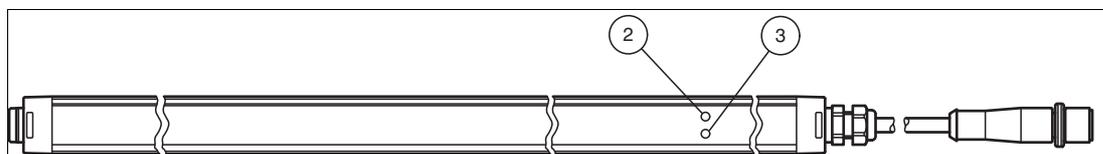
Figure 4.1 Function indicator on the emitter unit
