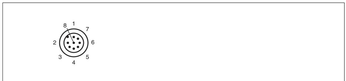
Figure 4.5 Receiver unit connection layout
